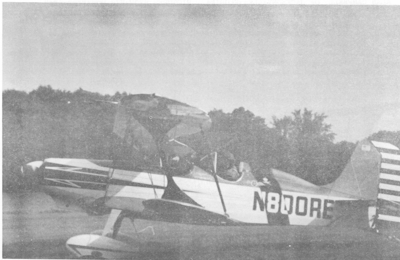
STARDUSTER TOO BY FRANK HOSTERMAN, 1000 STAFFORD STREET, MINERVA, OHIO, 44657 Engine is O-435 Lycoming---190 H.P.
