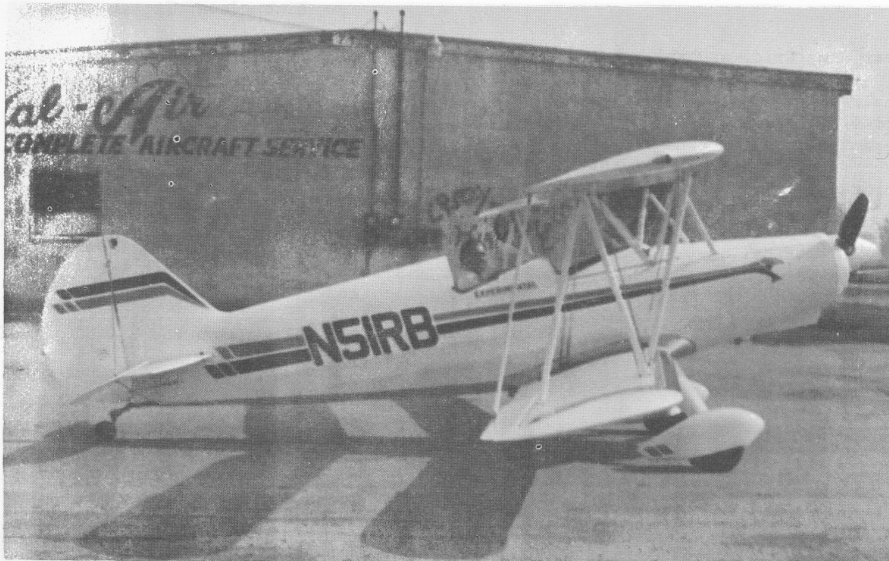
Our Good Friend, Roger Baumert, and his beautiful new Marquardt Charger. First Flight was made at Flabob Airport during June, 1977. Power is 150 H.P Lycoming.
