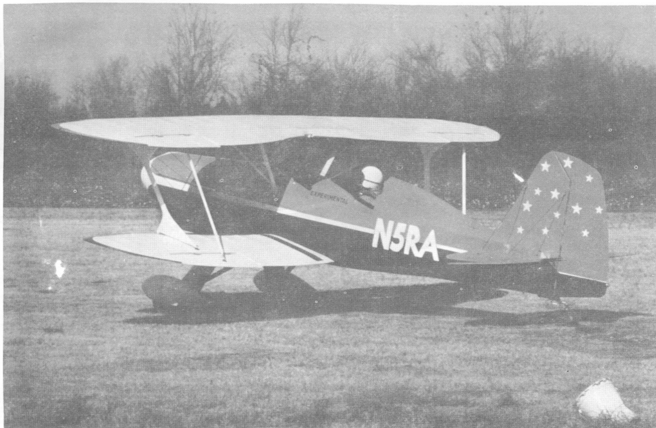
A BEAUTIFUL STARDUSTER TOO BY MR. ROBERT AUSTIN, OF HUNTSVILLE, ALABAMA POWERED BY 180 H.P. LYCOMING
