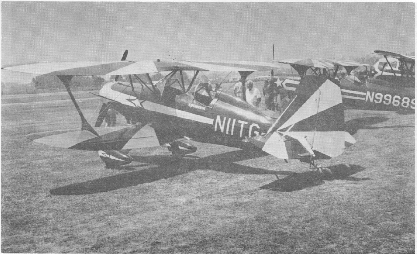
STARDUSTER TOO, BUILT AND OWNED BY TOM GREENE, OF HEMET, CALIF. THIS BEAUTIFUL BIRD HAS A 260 H.P. LYCOMING, AND EXCELLENT PERFORMANCE. PICTURED NEXT TO ED CARROL'S STARDUSTER TOO.
