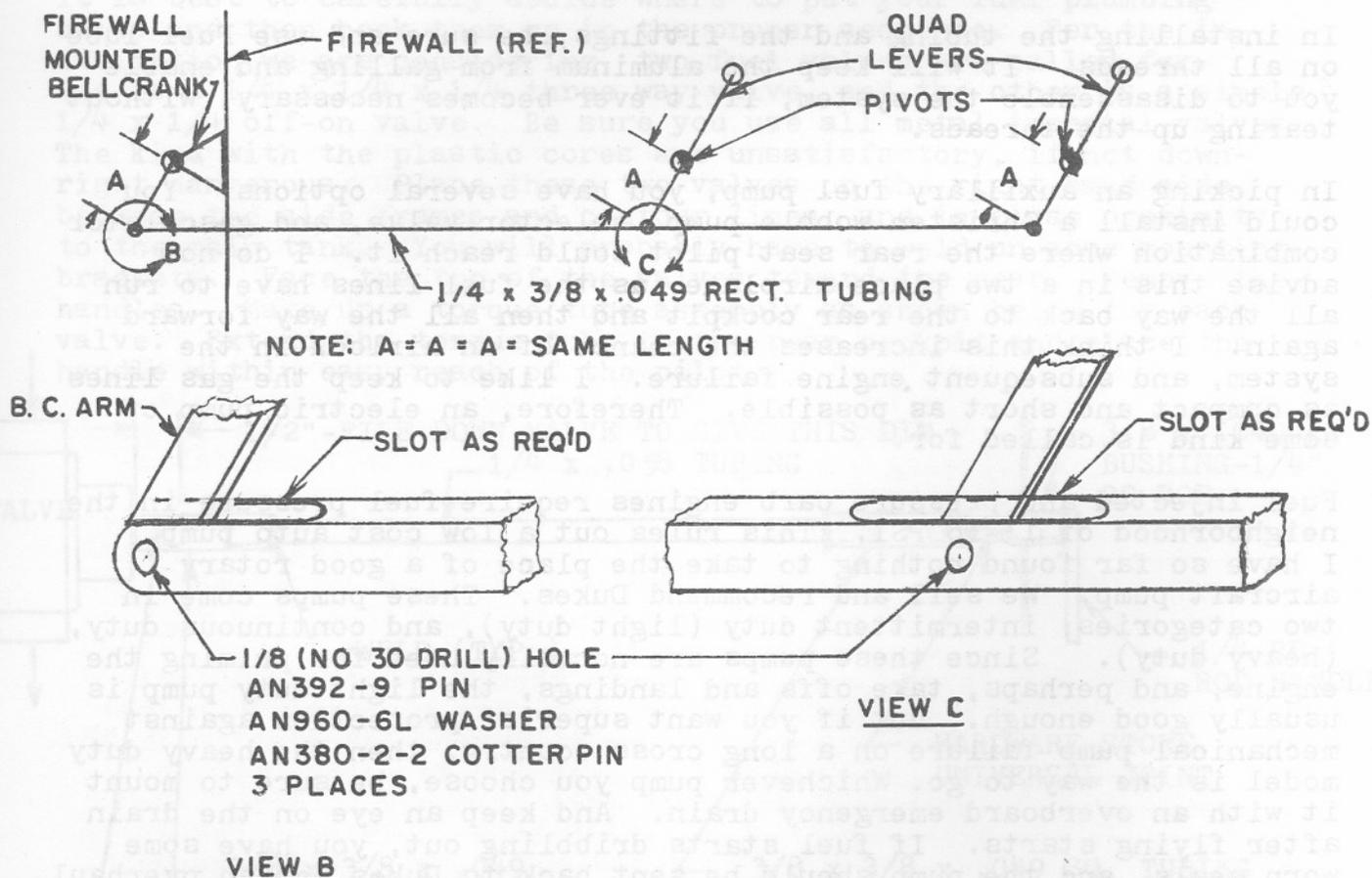
NOTE: THE RECTANGULAR TUBING IS ONE PIECE, AND RIGID- THEREFORE, ALL BELL CRANK ARMS MUST BE SAME LENGTH AND SAME ANGLE.
