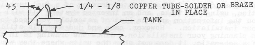
For venting the main tank, you must run two vent lines. On the top front of the tank there are three 1/4 pipe weld in fittings. The one on the right (pilots view) is the inverted vent. It goes clear to the bottom of the sump tank. Run 1/4" soft aluminum tubing from this fitting up the cabane strut, and terminate right under the wing. Have it face into the wind at a 45 degree angle.
