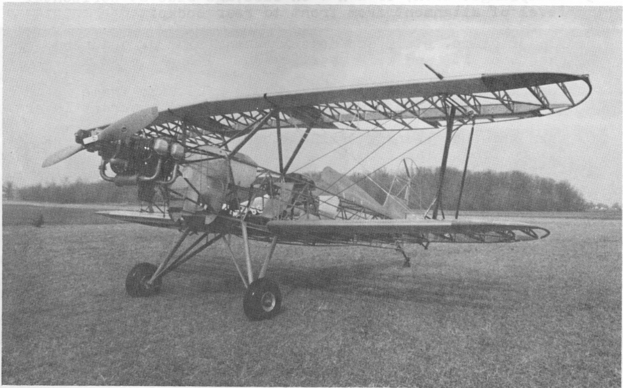
ABOVE IS NICE SHOT OF LESTER ZEHR'S STARDUSTER TOO. THE FIRST 90 % APPEARS TO BE DONE. THIS IS THE AIRPLANE WITH THE ENGINE TURNED STAINLESS STEEL FIREWALL.
