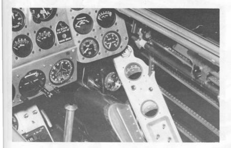
The instrument panel is tilted forward, with sides bent back. the 3 gyros can be pulled out as one unit.
