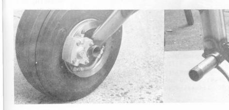
A special mounting bracket was made for the brake calipers and welded to the landing gear leg, allowing the axle to be shortened by 1 5/8 inches and placing the gear leg close to the inner wheel bearing.
