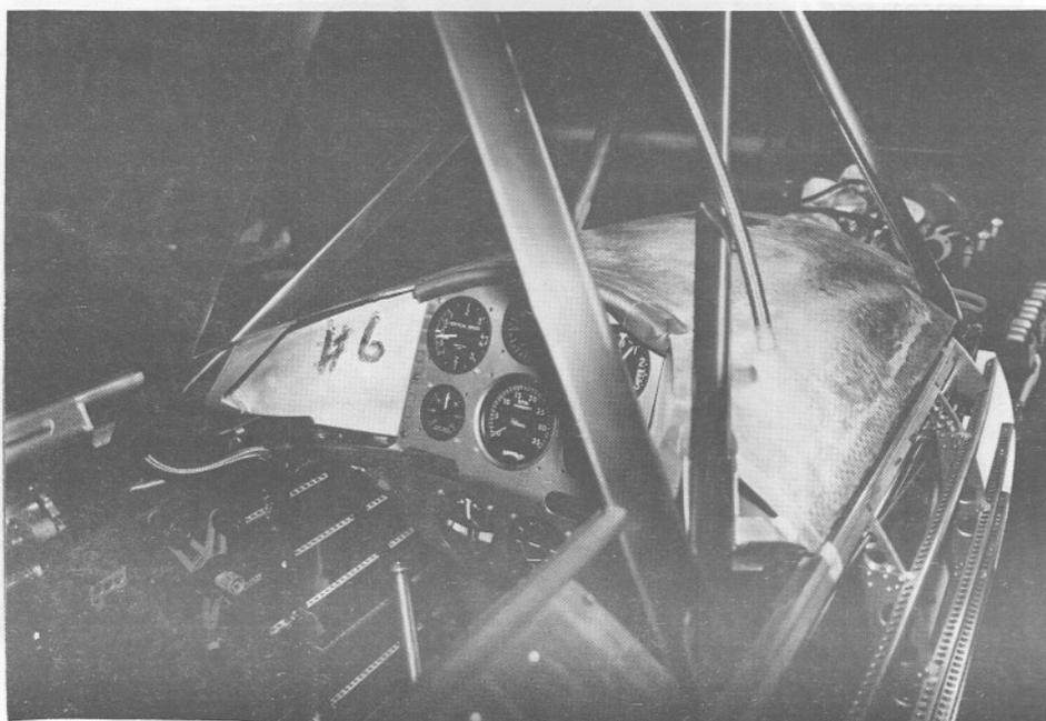
Not realizing at the time that it put the bottom rear of the tank past the cross piece of tubing on top of frame. By that time the rear of tank was welded in place. The front panel was held in place with duct tape, not yet rivited. (Lucky Me)
